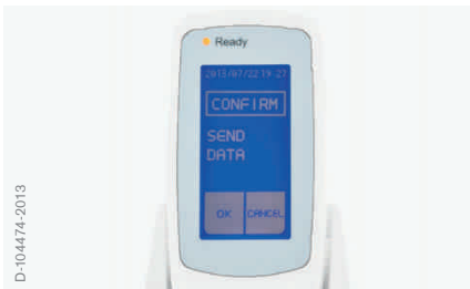
4. Nurse docks JM-105 into docking station, which is connected to the hospital network
